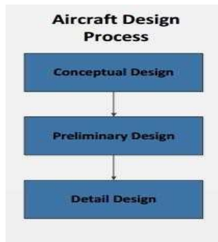
Fig.3. General Overview of Aircraft Design Process.
